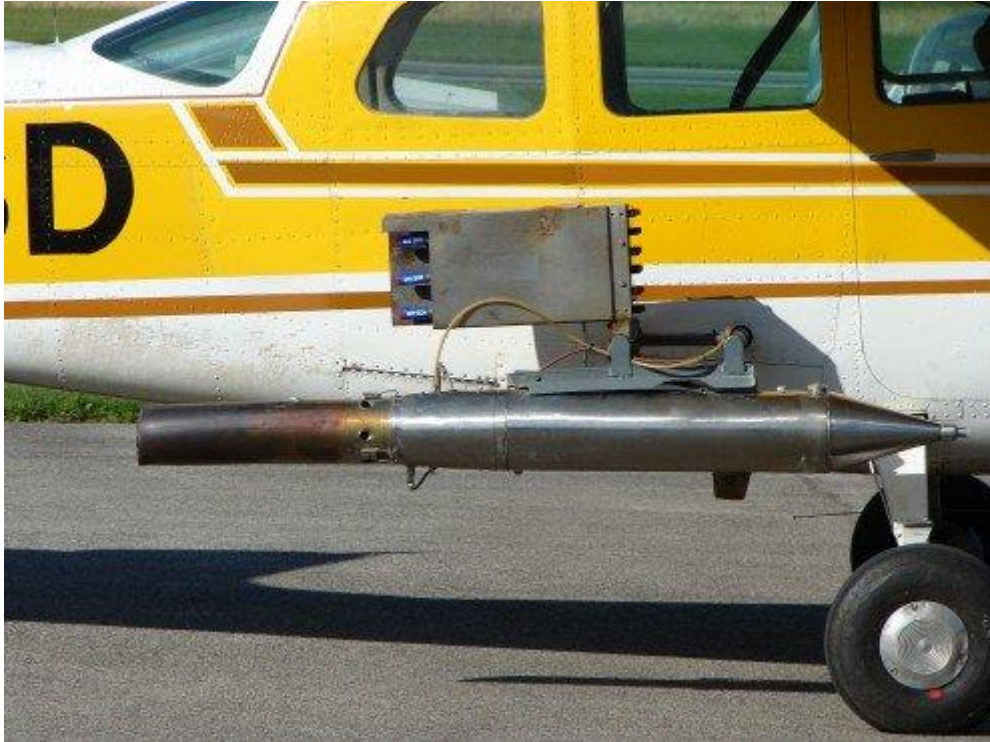
Air-Spraying Equipment - This is a wing mounted generator for spraying silver iodide. | Source
